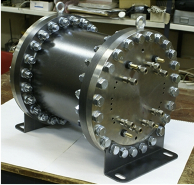
Figure 7.21 Photograph of a high-pressure bi-stack with its pressurization vessel.
