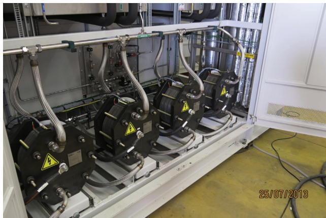
Figure 9.12 Photograph of a four-stack PEM water electrolyzer (courtesy of CETH Co.).
