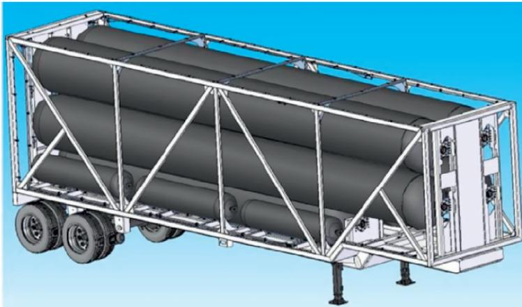
**Figure 13.1** US DOE's Lincoln carbon fiber composite tube trailer pressure (US DOE, 2012).
