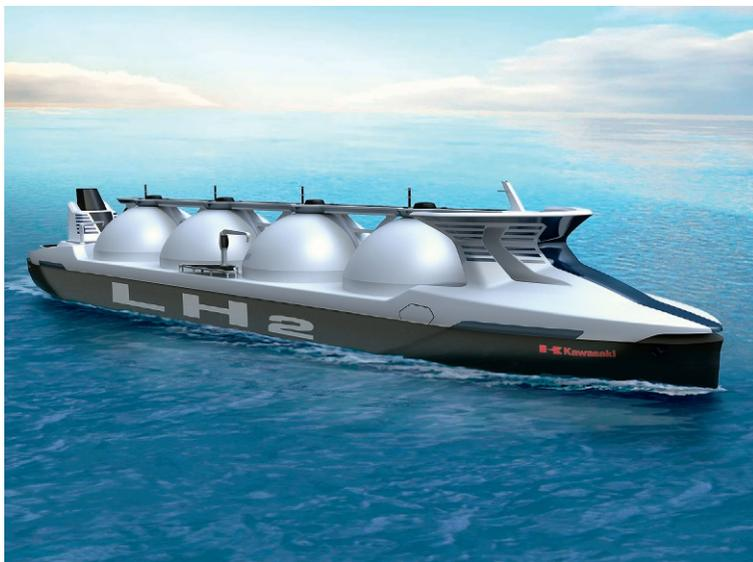
**Figure 11.4** Liquefied hydrogen carrier in a rendering by Kawasaki Heavy Industries, Ltd.
