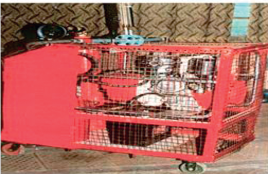
Hydrogen-fueled diesel engine
