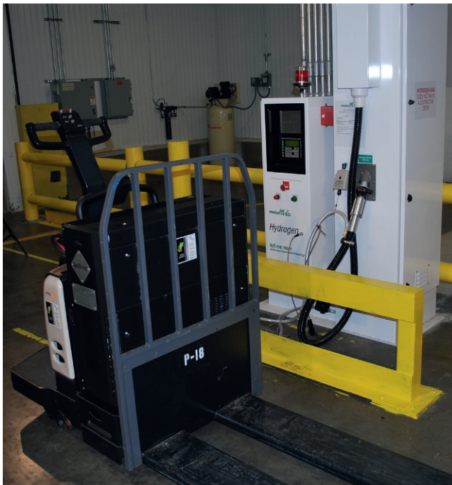
Figure 2.4 Fuel cell industrial truck refueling (Image courtesy of Air Products and Chemicals, Inc.).
