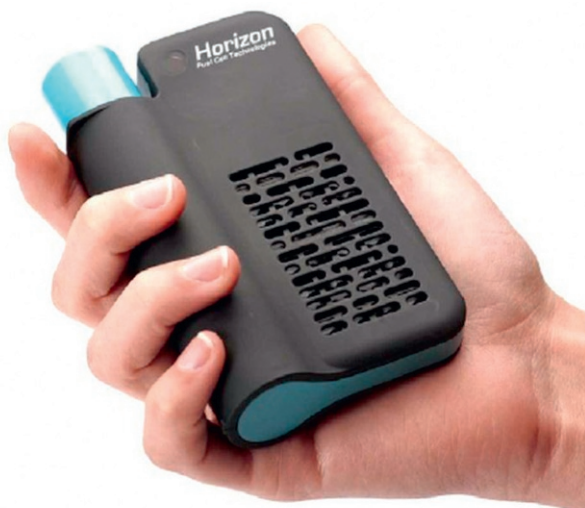
Figure 6.6 Horizon MiniPak fuel cell charger (Hart et al., 2014).
