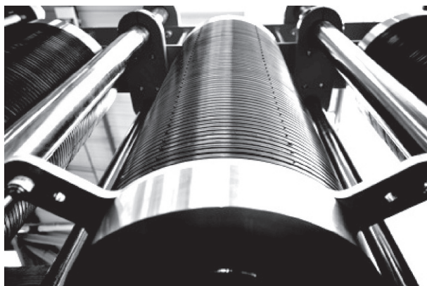
Figure 8.4 Self-pressurizing 80bar PEM stack. Courtesy of ITM Power plc.
